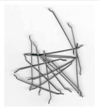
workable and the fibers are evenly distributed. Chemical admixtures or adjustments to the concrete mix design may be necessary to achieve proper consolidation and workability. It is important to follow the manufacturer's instructions on introducing the fibers into the mix and to closely adhere to safety precautions.
